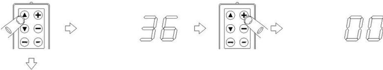
Function 'Time Setting Mode'. Press 'Up' to enter 'Time Setting Mode' and set the seconds count.
