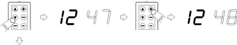
Seconds Setting Mode. Press '+' to increment seconds, '-' to set to zero. Press 'Up' to set minutes count.
